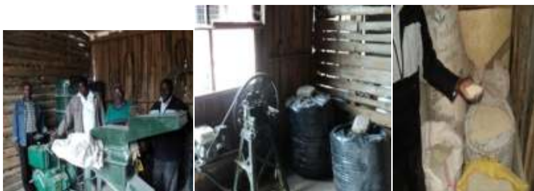
Plate 2: A 20HP chopper grinder motorised chaff cutter and processed silage
